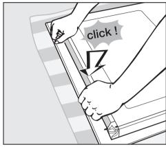
■ Finally using the ball of your hand press down on the aluminium trim on the inner pane to make sure it goes back into position. You will hear a very clear "click" when doing this. The retaining pins are pushed back out when you do this.
